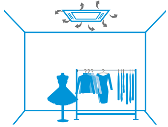
Air distribution with a dusty filter
