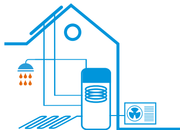
Floor standing unit with integrated ECH 2 O tank
